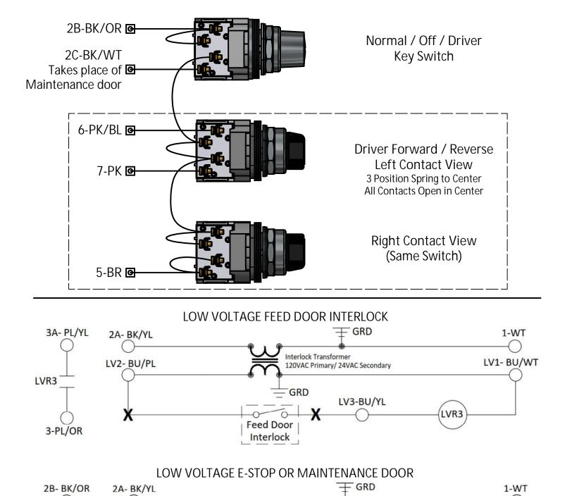
"X" indicates interlock plug. "LV\_" are additional low voltage terminal blocks.
