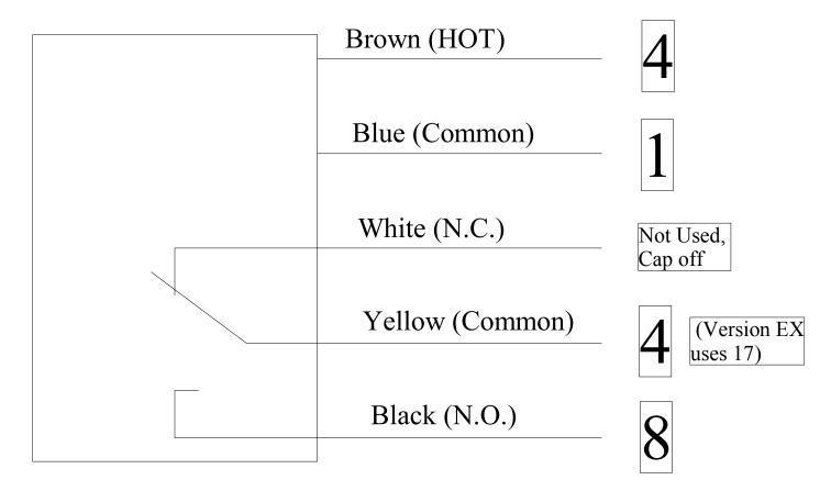
Note: Unlike our other eyes, this photo eye uses a reflector. The range is 6" to 20'. Also, this eye should be set on "D/O". To change from L/O to D/O, open the cover and flip the switch.
